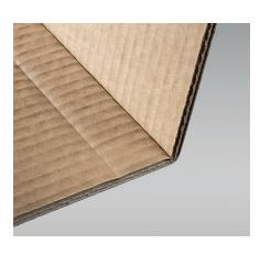
The CTT3 is designed for processing double-wall corrugated card-board. The tool accommodates crease wheels with a diameter of 90 mm and a width of 28 mm. With or across the corrugation, these crease wheels ensure high-quality results without damage to the top layer. The wheels snap into the holder, making them quick and easy to insert
