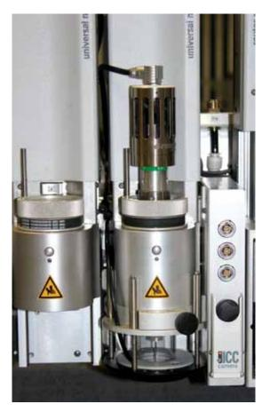
Used in the processing of prismatic, reflective materials for emergency traffic fleets and road signs where high conspicuity is essential. The Sonicz tool uses a specially developed range of tooling to cut and edge seal the reflective materials in a single cutting pass giving a guaranteed seal and longevity to the finished product.
