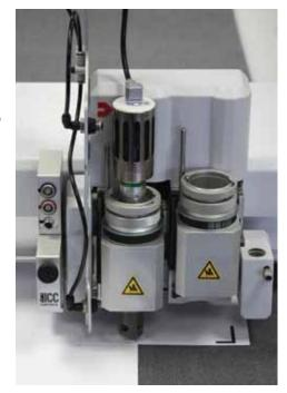
In applications where sealed or finished edges is a prerequisite, the Sonicz tool in combination with the cutting surface will offer a solution.
