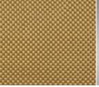
Aramidfiber Kevlar™ woven, knitted, or uni-directional textile structure. Single and multi- gle or multi-ply.
