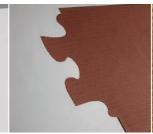
Prepreg pre-impregnated fiber. Semi-finished product of carbon or glass fibers and a non-hardened duro- or ply. thermoplastic matrix.
