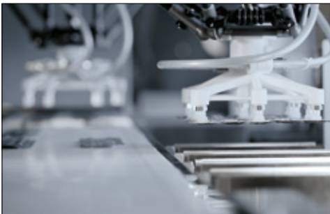
Robot feeding system for single or multiple strips
