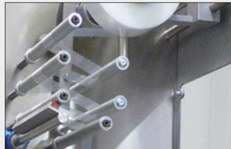
Strain release during foil unwinding
