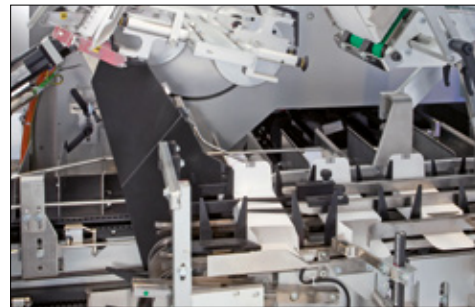
Carton positive opening and product feeding into cartons
