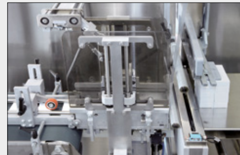
Stacking unit and hot sealing bar
