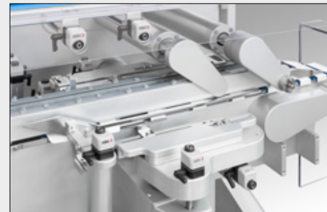
Positive carton transport by top and bottom guides
