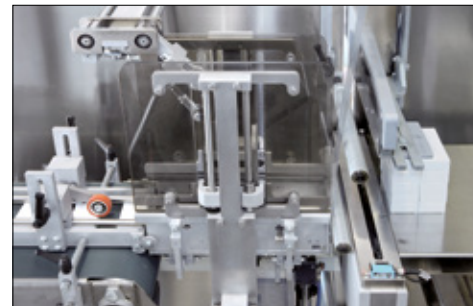
Stacking unit and hot sealing bar
