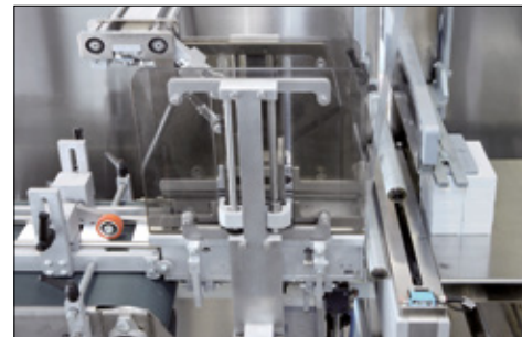
Stacking unit and hot sealing bar
