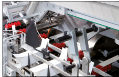
Product feed into the open cartons
