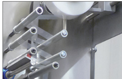
Strain release during foil unwinding
