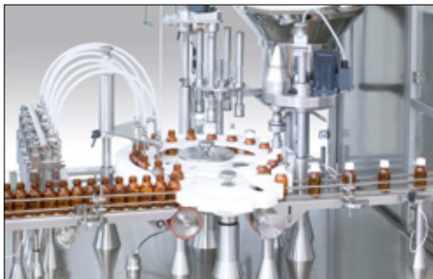
Transport systems by starwheels
