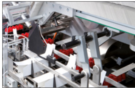
Product feed into the open cartons
