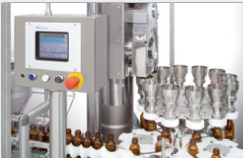
Powder filling station
