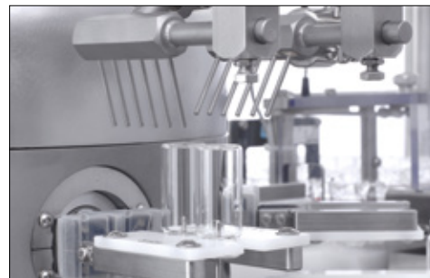
Internal and external cleaning station
