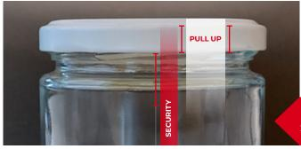
**PULL-UP:** distance in mm between lines 2 & 3 **SEAL SECURITY:** distance in mm between lines 1 & 2
