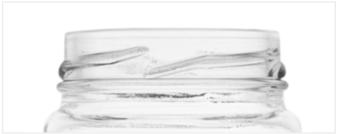
Helical thread without stop function, special for his double slant. Usually only for closure diameters 43mm - 48mm. This double incline helps screwing-on and avoids over tightening.
