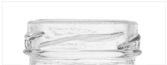
It is the "stop" finish, indeed its thread has, at the end of central horizontal segment, a real angle that impedes to screw on further. It is used usually in small diameters, up to 43 and 48mm.
