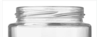
Helical thread without stop function (angle). Closure lugs progressively tighten, under the thread, while twisting on. A classic example is finish T.O. 82 FD 130 of item 10145 P2 V ORTO 580 T 82 PG.
