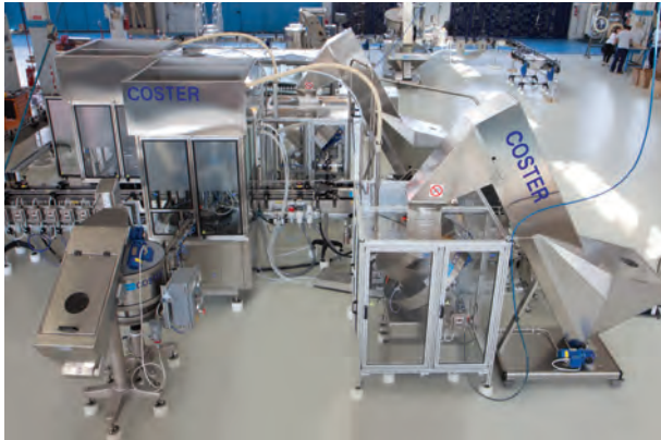
Above, machines for liquid filling: sorters for two different types of valves; Valve Crimping, on a back to back configuration.
