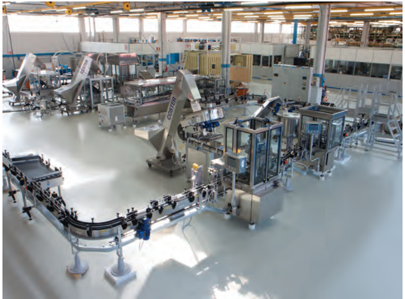
Above, machines for liquid filling: sorters for two different types of valves; Valve Crimping, on a back to back configuration.
