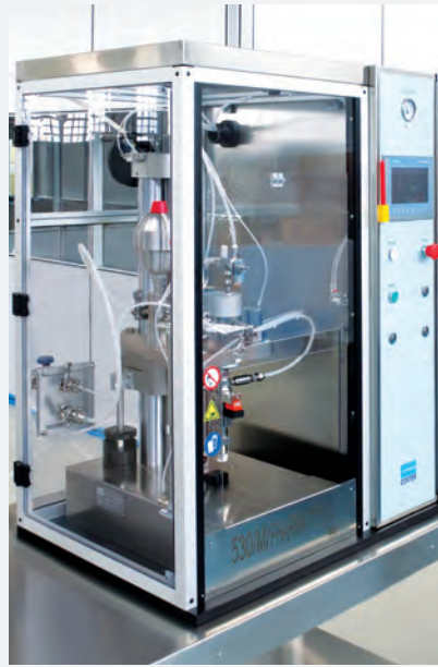
Left, vacuum and valve crimping on 530/S/V/20C-PHARMA semiautomatic machine.
