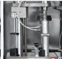
500D semiautomatic machine for filling into open can liquid products with a maximum viscosity of 1000 cp. The machine, completely pneumatic, is able to operate on one or two cans at a time (depending on the number of metering cylinders installed), with the possibility of receiving cans with diameters ranging from 35 mm to 66 mm and heights ranging from 75 mm to 300 mm.
