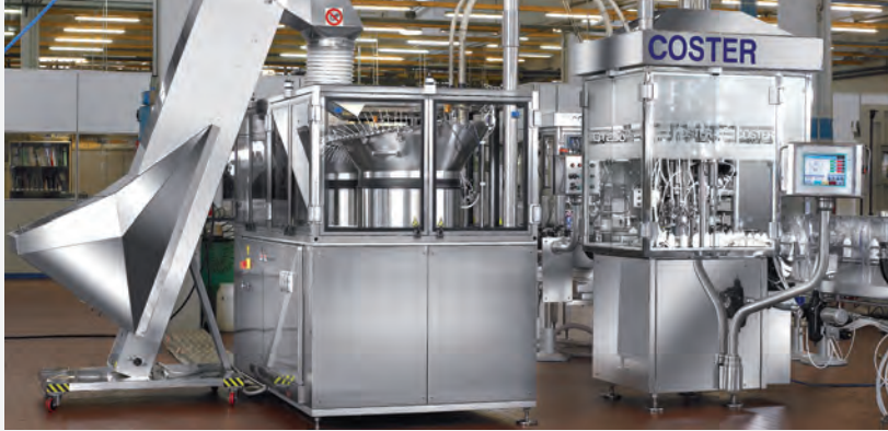
Left, double indexing 1" aerosol valves filling line. Speed up to 90 cpm.
