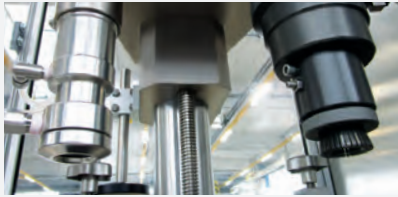
Left, vacuum and valve crimping on 530/S/V/20C-PHARMA semiautomatic machine.
