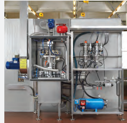
Left, double indexing 1" aerosol valves filling line. Speed up to 90 cpm.
