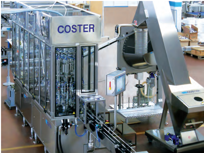
Left, double column rotary machine for liquid filling, valve insertion and crimping.
