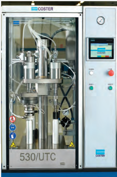
Left, 530/UTC unit for pressurized crimping of Bag On Valves.
