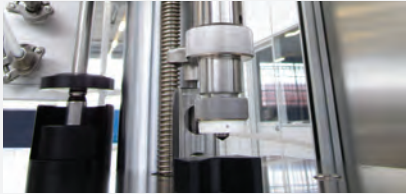
Left, vacuum and valve crimping on 530/S/V/20C-PHARMA semiautomatic machine.
