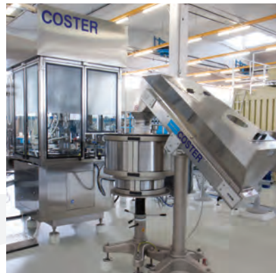
Left, valve feeder.
