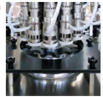
Left, double column rotary machine for liquid filling, valve insertion and crimping.
