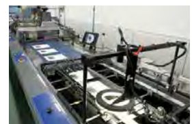
Our Attacher System, which automatically attaches and packs thin samples.
