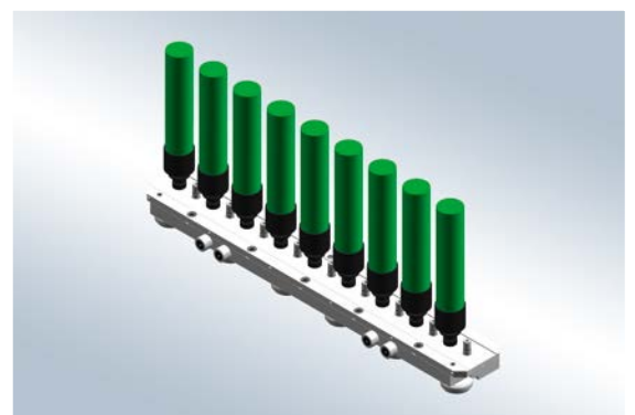
Carrier equipped with 9 substrates, up to 5,450 parts/h
