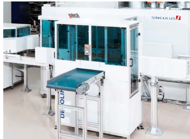
Unloading station directly after top coating
